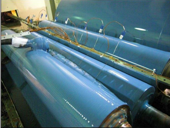
Figure 14: Measuring Temperatures in a Roll Coating System
